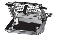
**4** Use a soft cloth to gently wipe the scanner glass on the top (A) and the white strips on the bottom (B).
