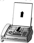
**2** Open the operation panel by lifting in the middle. When you hear a soft click, the panel is engaged.
