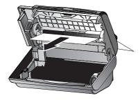
**4** Turn small roll forward to tension the ink film. Make sure that the ink film is not creased.
