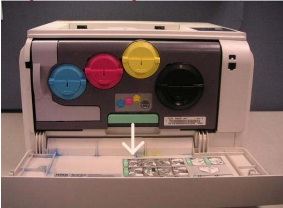
2. Remove InterTransfer Belt Unit by grasping bottom of ITB and pulling out slightly until it releases, lower it slightly, and continue pulling out to remove ITB. NOTE: Observe removal path for, especially rear of ITB for reinstallation. **CAUTION: Do not touch the ITB Belt. Protect it from light.**
