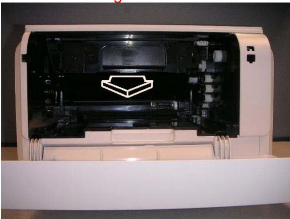
3. Remove Screws (2) and remove Top Cover by lifting the front of the cover slightly and pulling forward to release hidden clips at under rear of cover.
