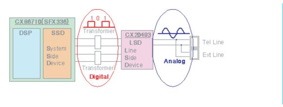
Transformer transfer Clock from SSD to LSD and Clock Frequency is 4.032MHz.
