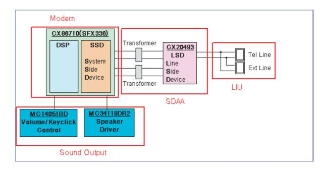
Implemented by based on Conexant DAA (Data Access Arrangement) Solution, and is roughly composed of two kinds Chip Solution
