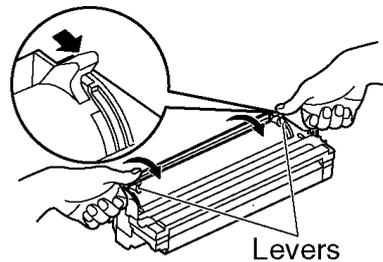
11. The toner cartridge is installed when the triangles match.
