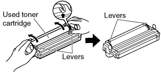
6. Pull up the right edge of the used toner cartridge (①). Remove the cartridge from the drum unit (②).
