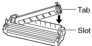
9. Firmly press down on the right side of the toner cartridge to snap into position.
