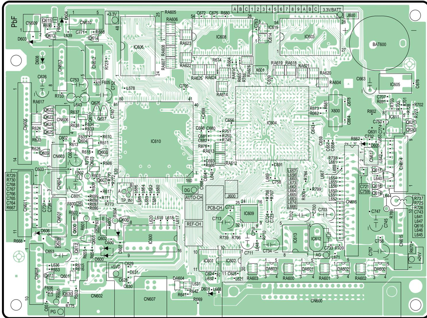
KK-FLB758EX DIGITAL BOARD (PCB1) COMPONENT VIEW
