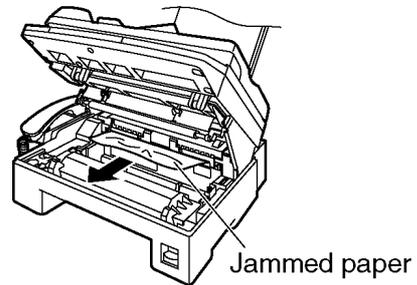
**When the recording paper has jammed near the recording paper exit:**
