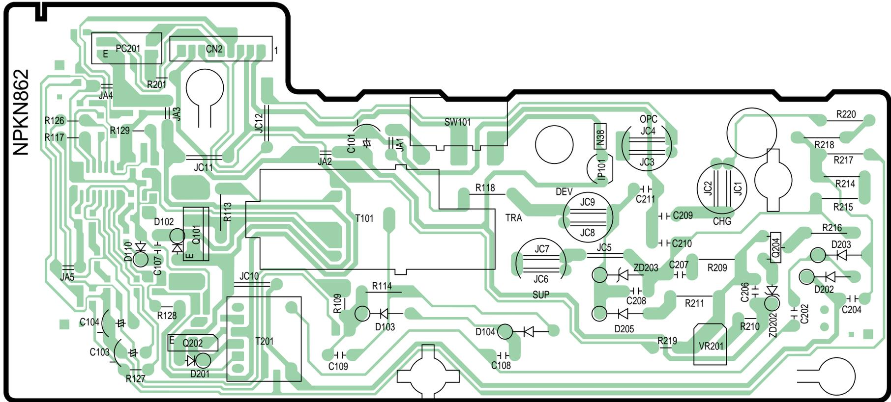
KX-FLB758EX HIGH VOLTAGE POWER SUPPLY BOARD (PCB4) COMPONENT VIEW
