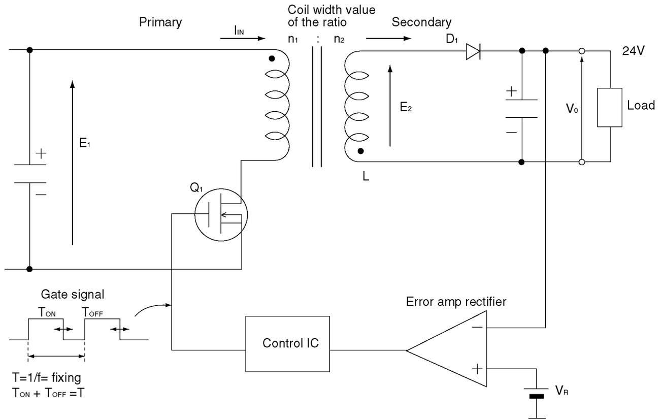
The following is an overview of how the power supply unit is controlled.
