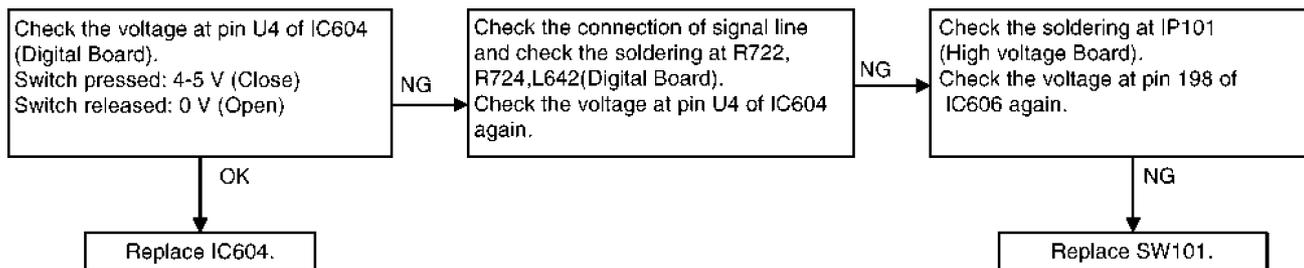
**5. Check the DRUM sensor..... “CHECK DRUM”**
