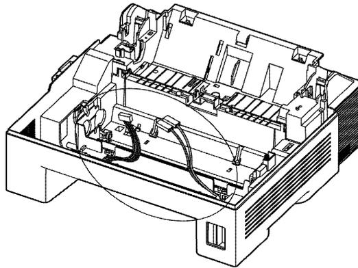
After connecting Fusser lead wire, pass the brown wire first and the black wire next in between the rib and the wall.
