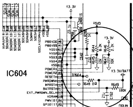
When the Reset signal indicates 'H', check the items below.
