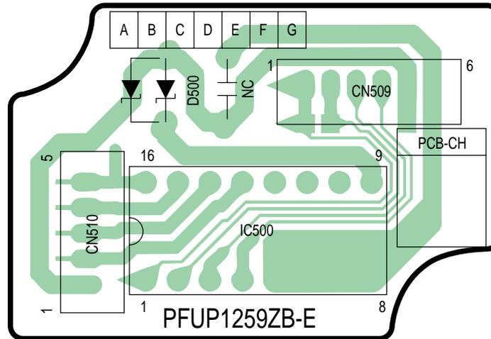
KX-FLB758EX SCAN MOTOR DRIVER BOARD (PCB13)
