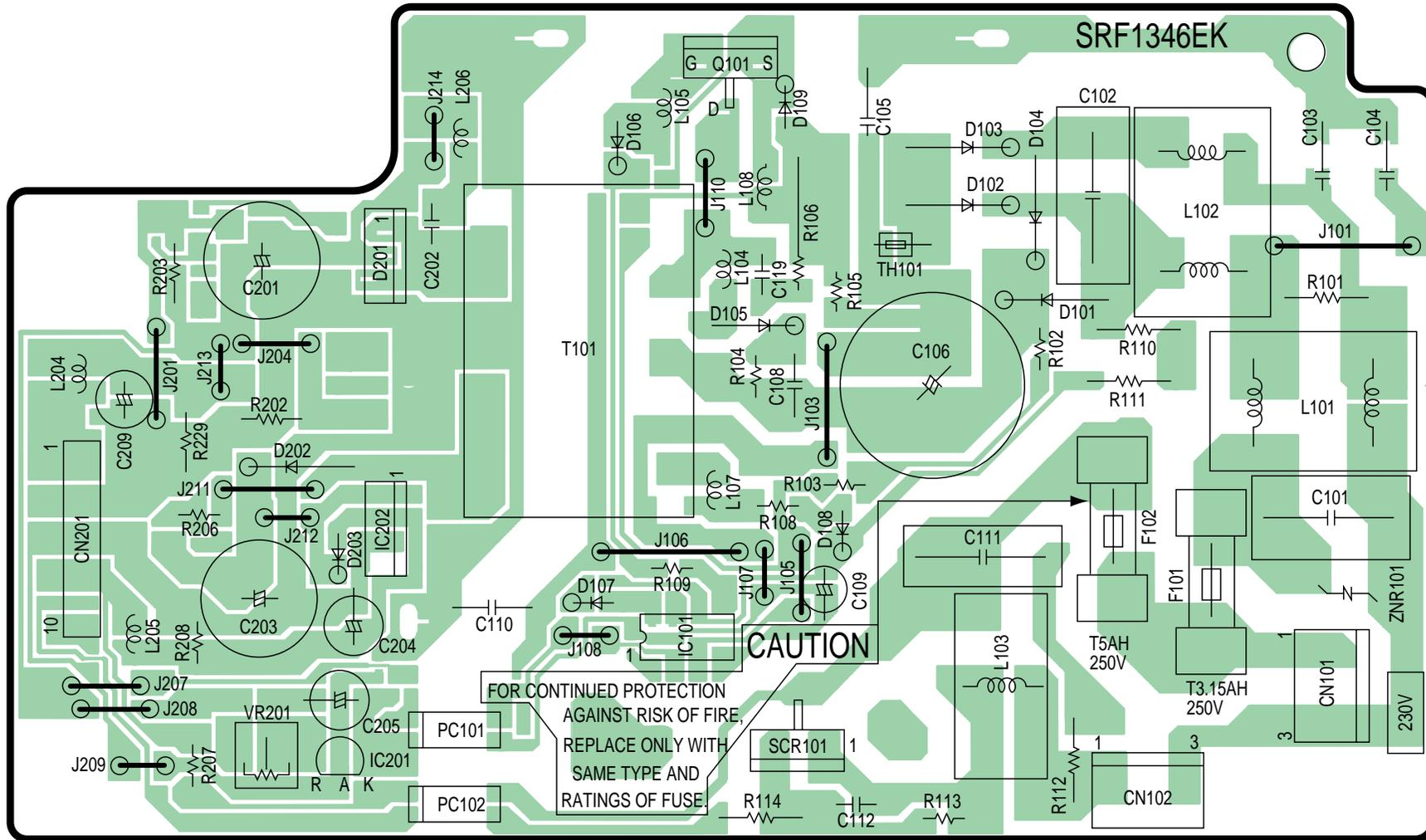
KX-FLB758EX LOW VOLTAGE POWER SUPPLY BOARD (PCB5) COMPONENT VIEW
