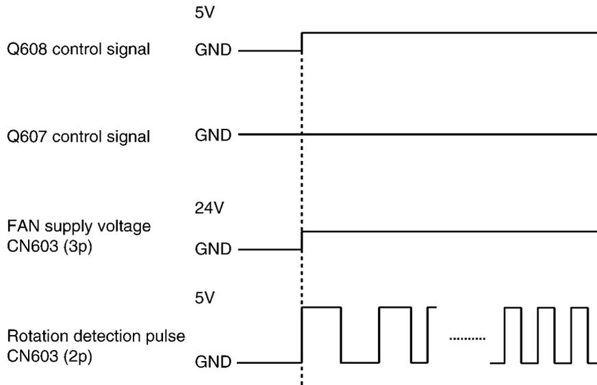
2. Low-speed rotation (typ. 2400 rpm)
