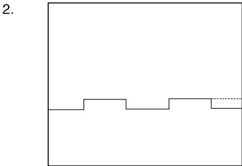
Short between the signal line and GND.
