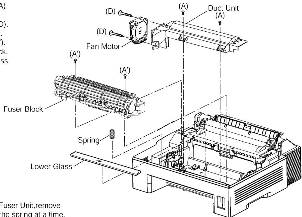
Note: When removing the Fuser Unit,remove the lower glass and the spring at a time.
