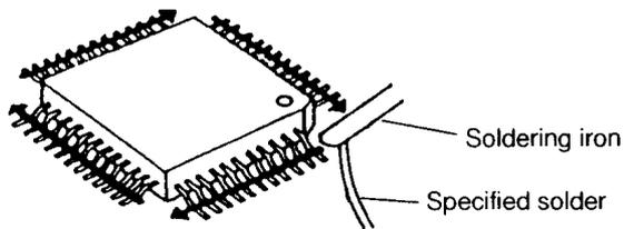
Be certain each pin is located over the correct pad on the PCB.
