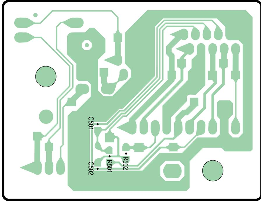
KX-FLB756EX CIS RELAY BOARD (PCB11) BOTTOM VIEW
