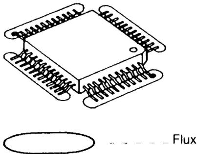
3. Being careful to not unsolder the tack points, slide the soldering iron along the tips of the pins while feeding enough solder to the tip so that it flows under the pins as they are heated.
