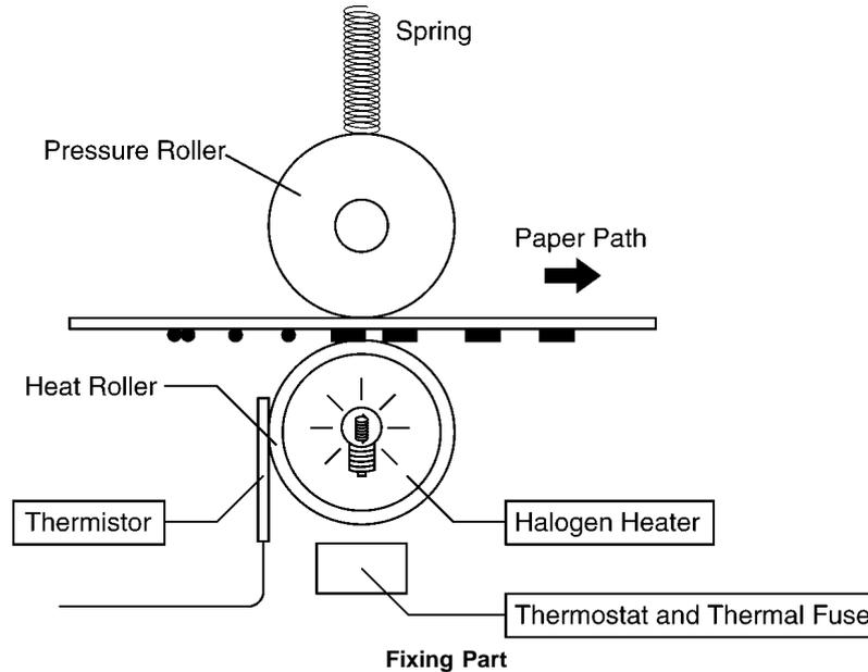
The fixing part becomes high temperature, so the thermistor and the thermal fuse are provided.
