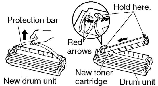
8. Slide the tab on the toner cartridge into the slot of the drum unit.
