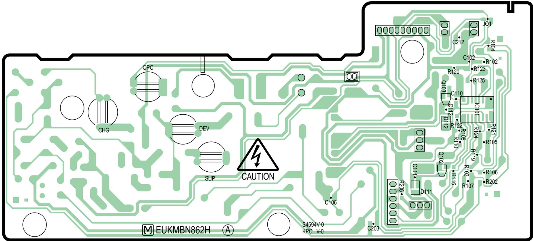
KX-FLB758EX HIGH VOLTAGE POWER SUPPLY BOARD (PCB4) BOTTOM VIEW
