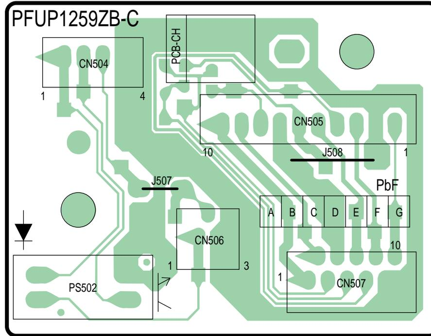
KX-FLB758EX CIS RELAY BOARD (PCB11) COMPONENT VIEW
