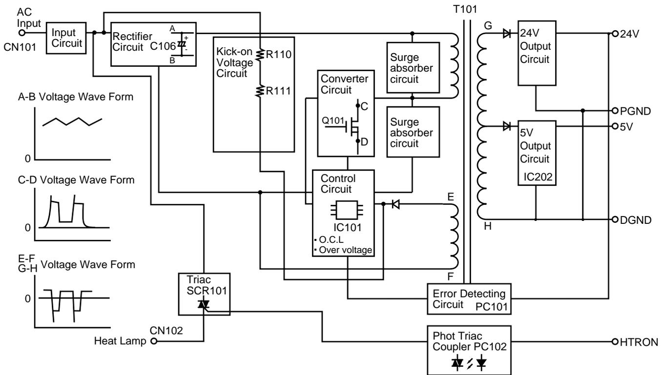
KX-FLB758PD: POWER SUPPLY BOARD: BLOCK DIAGRAM
