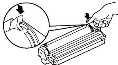
10. Turn the two levers on the toner cartridge with firm pressure.
