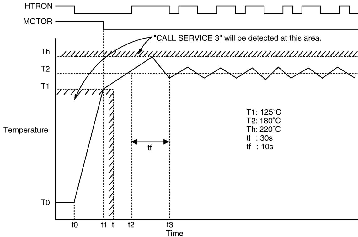
T0: Initial Temperature (At Power OFF / Normal Temperature)
