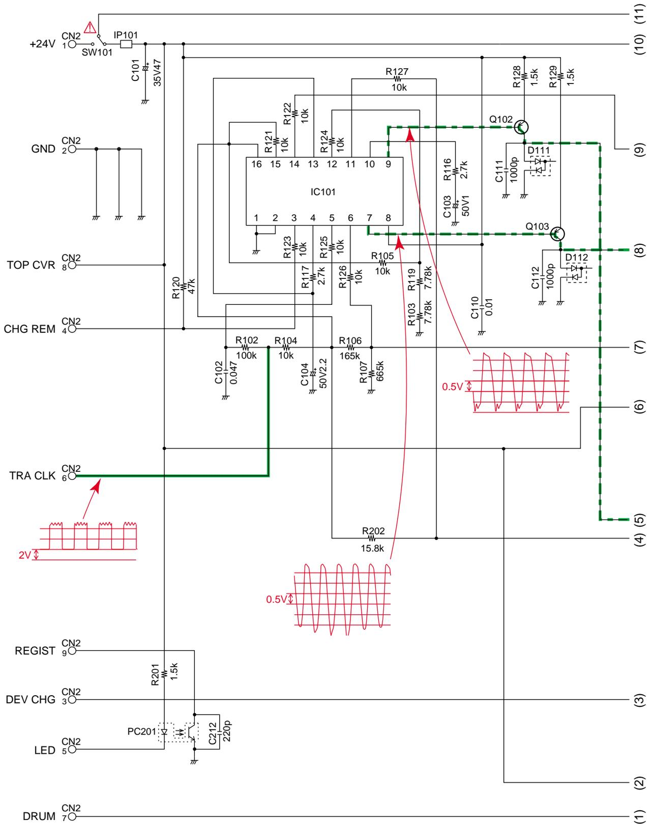
KX-FLB758EX HIGH VOLTAGE POWER SUPPLY BOARD (PCB4) 1/2
