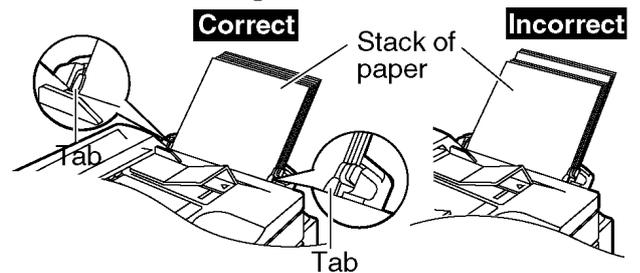
4. Adjust the width of the guides to the size of the recording paper by sliding the right recording paper guide.
