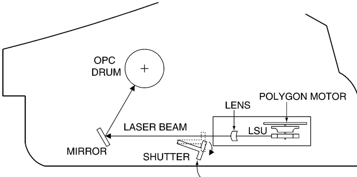
The mechanical shutter will be opened by setting DRUM UNIT properly.
