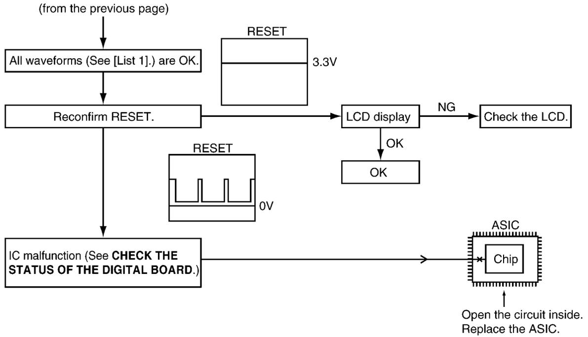
Other NG examples while the power is ON and the LCD displays the following.
