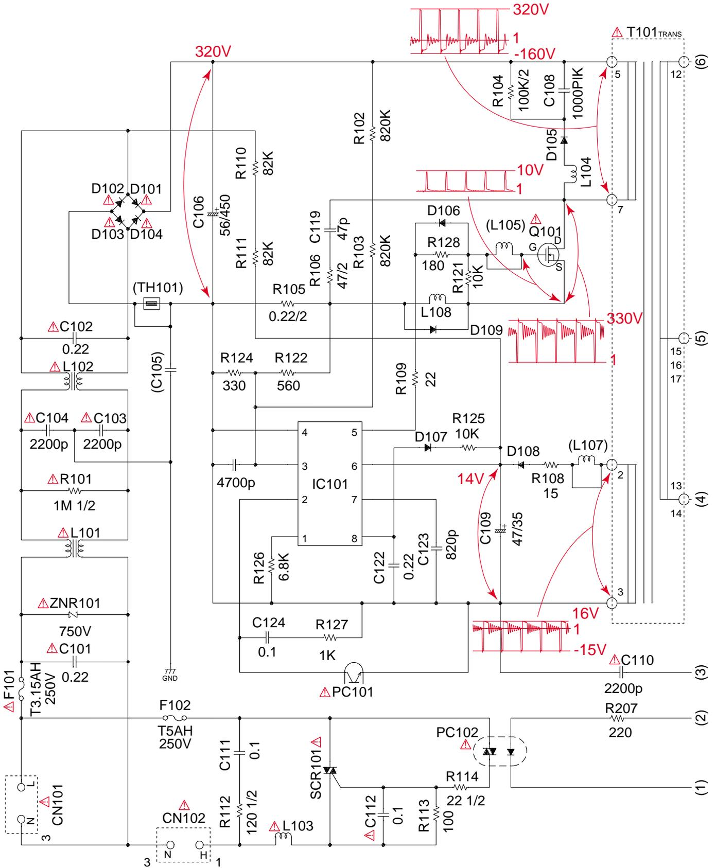
KX-FLB758EX LOW VOLTAGE POWER SUPPLY BOARD (PCB5) 1/2
