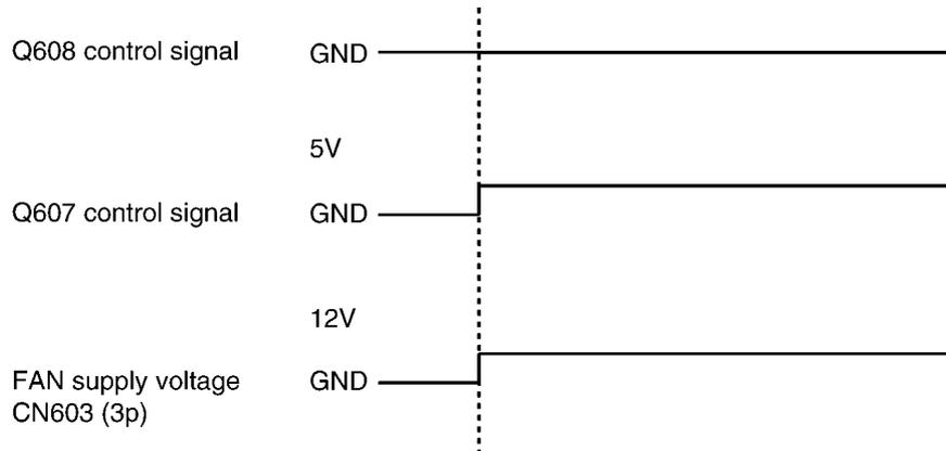
During low-speed rotation, the rotation detection does not function.
