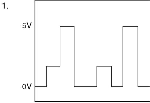
Short circuit from the adjacent signal wires.
