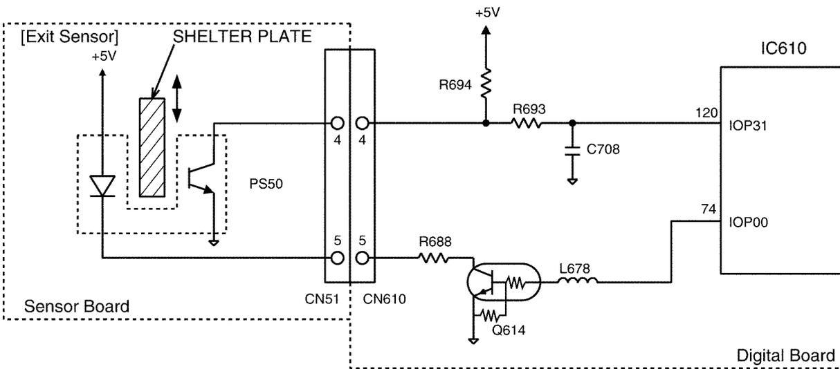
The sensor detects whether the recording paper exit out or not.
