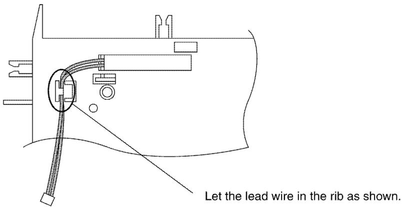
**Placing the lead wire of FUSSER UNIT.**
