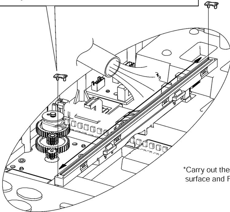
\*Carry out the air suction of the CIS reading surface and FB base surface fully.
