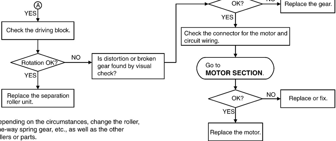
Depending on the circumstances, change the roller, one-way spring gear, etc., as well as the other rollers or parts.
