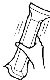
2. Remove the new toner cartridge from the protection bag. Peel off the seal from the toner cartridge.
