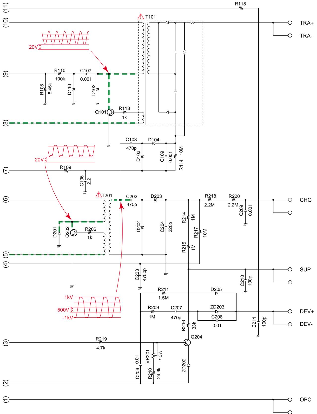
KX-FLB758EX HIGH VOLTAGE POWER SUPPLY BOARD (PCB4) 2/2
