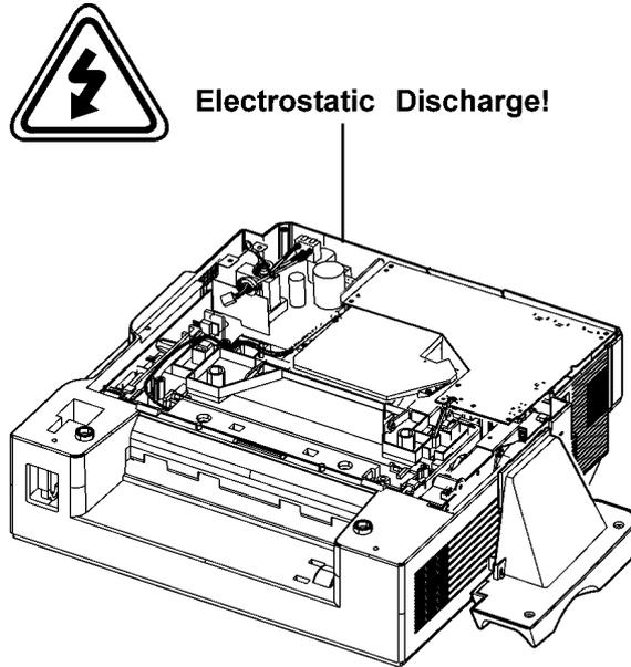
To prevent static electricity damage to the interface connectors (parallel and USB) or other electrical components inside the unit, touch a grounded metal surface, such as the metal part under the parallel interface connector before touching the components.
