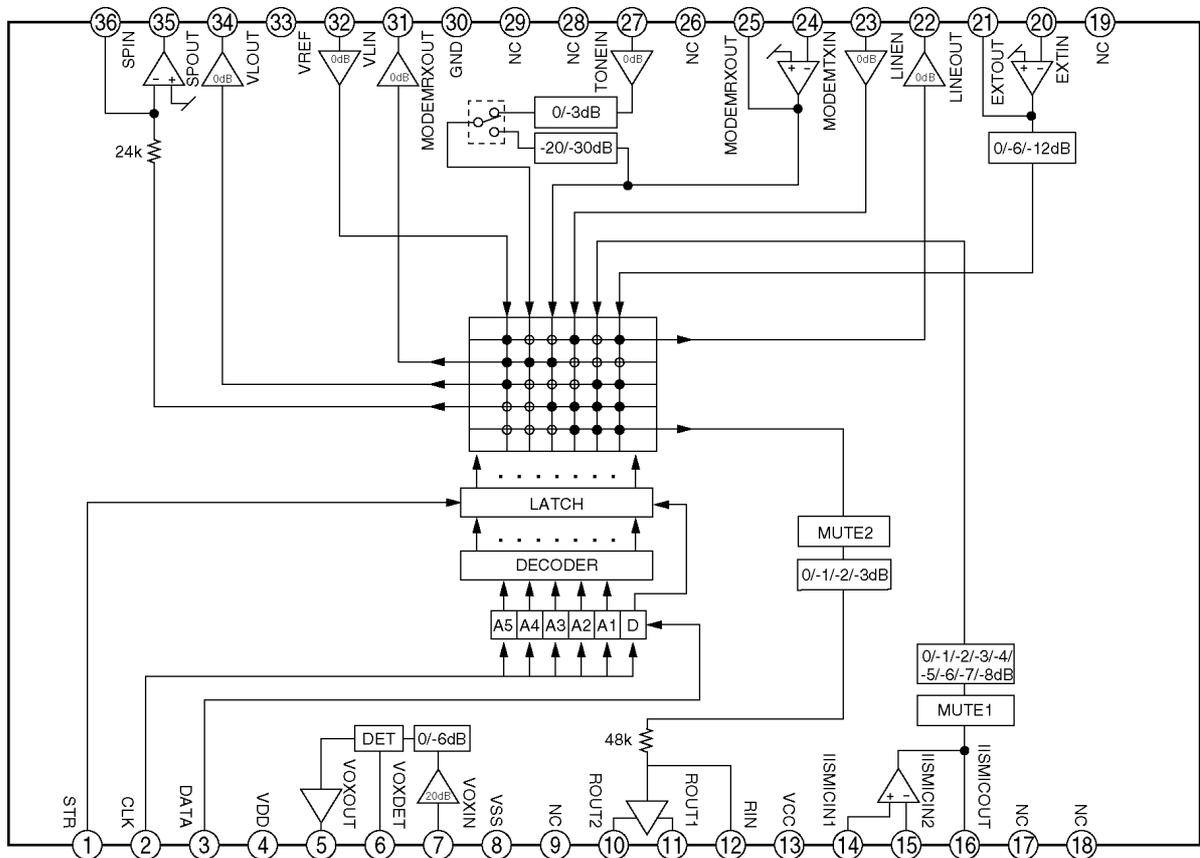
Explanation of ANALOG GATE ARRAY (IC201 on the DIGITAL Board)
