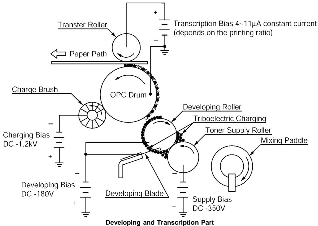
The values of developing bias and supply bias are different from the ones described in the Service Manual for FL501. The biases output from the unit of FL501,FLM551 and FLB751 (FLB750) have the same voltage. However, the developing device of FA78X(FA78A) converts the developing and supply biases inside the developing device to improve the image quality.
