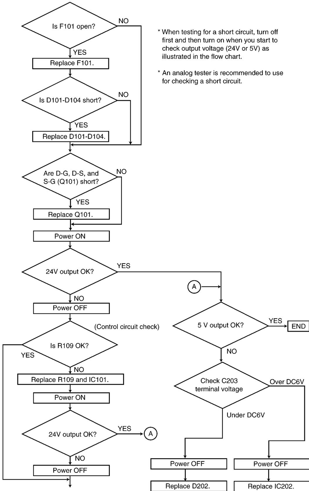
\* When testing for a short circuit, turn off first and then turn on when you start to check output voltage (24V or 5V) as illustrated in the flow chart.
