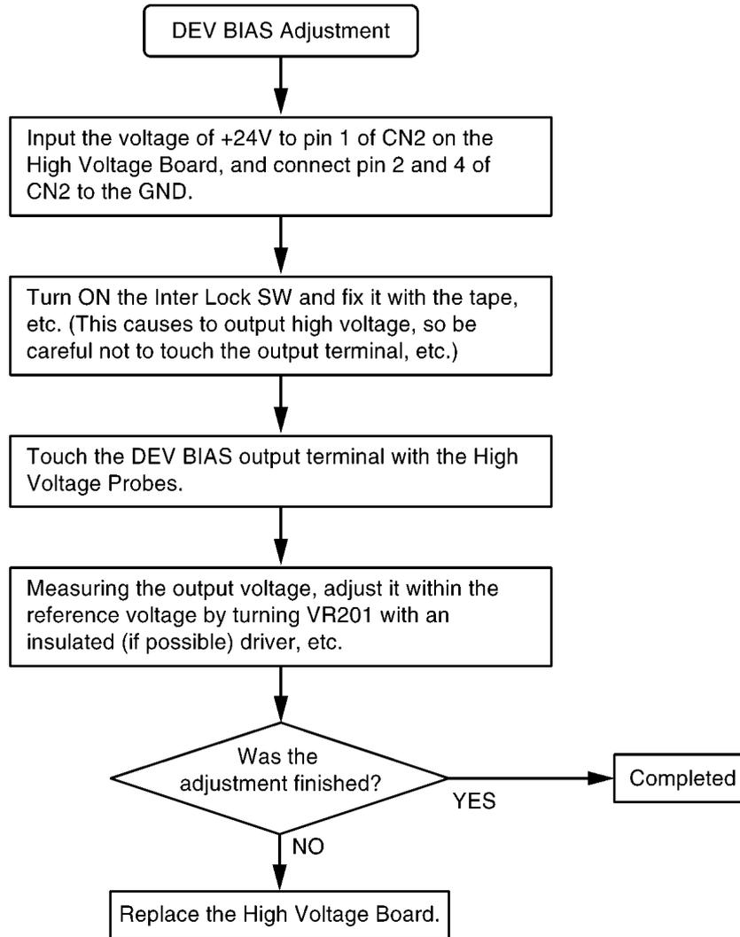
\* This Adjustment should be done with a single High Voltage Board.
