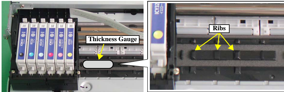
Figure 3-7. Setting Thickness Gauge
