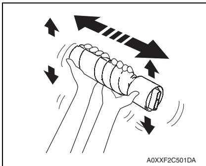
4. Remove the new toner bottle from its packaging, and shake it side to side 5 to 10 times.
