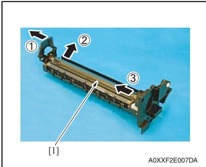
4. Remove the drum charge corona [1] as shown in the illustration.
