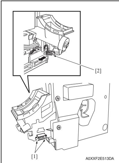
3. Release the tabs [1] and disconnect the connector [2] from the imaging unit.
