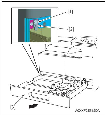
2. Remove the screw [1], and remove the fixed sheet metal [2].
