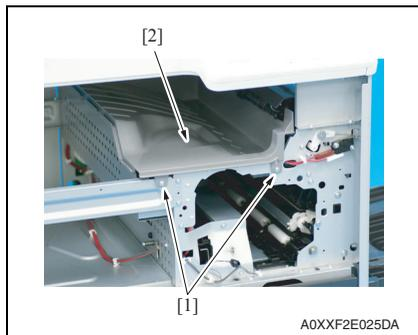
4. Remove two screws [1], and remove the paper exit tray (left) [2].
