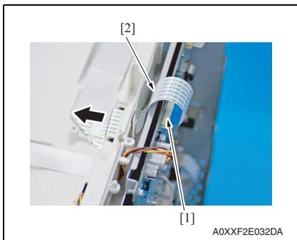
3. Disconnect the connector (P102) [1] on the printer control board.
