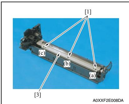
5. Remove three screws [1], and remove the cleaning blade [2].
