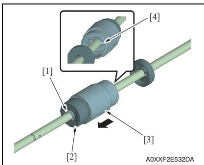
7. Remove the E-ring [1], and remove the weight [2].
