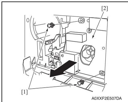
7. Remove two screws [1], and remove the imaging unit [2].
