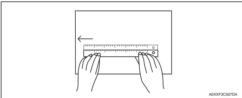
2. Measure the length of the scale on the copy. If the amount of error falls outside the specified range, perform the following steps to make an adjustment.
