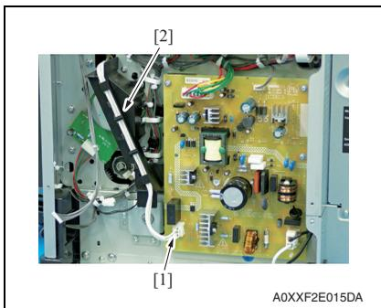
2. Disconnect the connector (CN2) [1] on the DC power supply.
