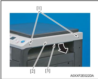
1. Remove two screws [1], and remove the scanner right cover [2].
