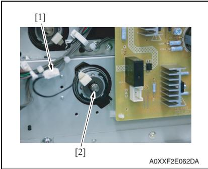
5. Disconnect the connector [1], and remove the tray paper feed clutch [2].
