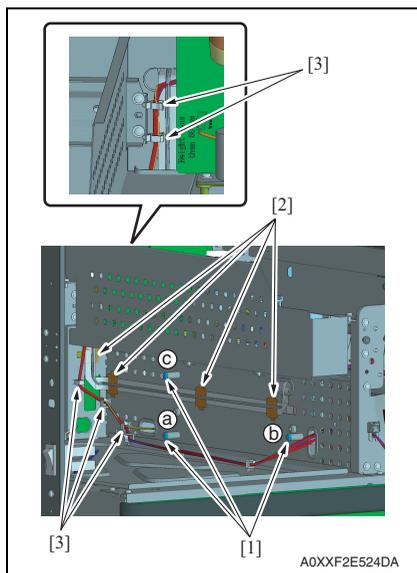
8. Remove three screws that have a spring [1].
