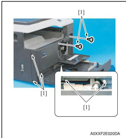
5. Remove seven screws [1], and remove the front cover [2].
