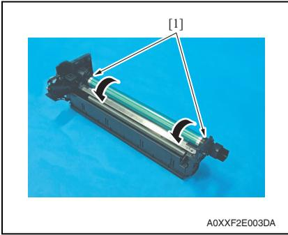
10. While turning the drum [1] in the direction of the arrow, dump the remaining developer from the screw.
