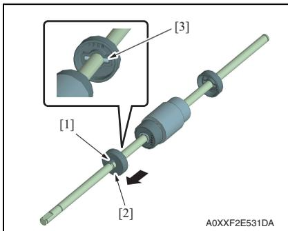
6. While releasing the tab [1], remove the collar [2].
