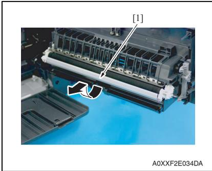
2. Remove the transfer roller unit [1] as shown in the illustration.
