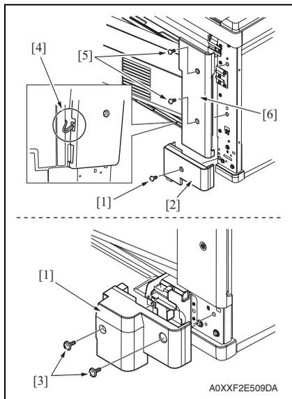
1. Remove the screw [1], and remove the rear right cover/1 (lower) [2].
