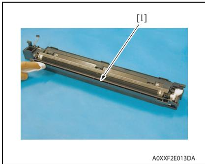
2. Using a cleaning pad dampened with alcohol, wipe the timing roller [1] clean of dirt.
