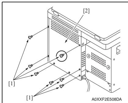
1. Remove seven screws [1], and remove the rear cover [2].
