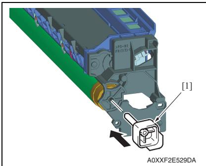
1. With the imaging unit divided into the drum assy and developing assy, install the drum positioning jig [1] in the rear of the drum assy.
