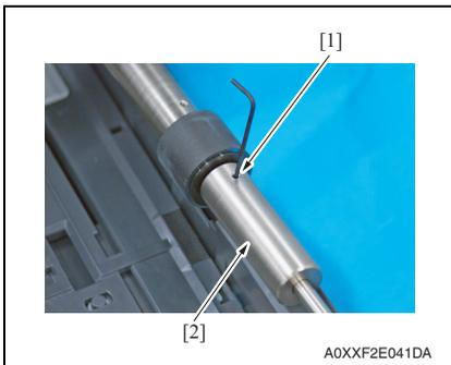
5. Loosen the set screw [1] with the hexagon wrench (2.5 mm), and remove the weight [2].
