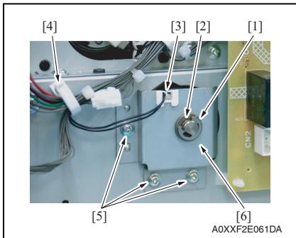
2. Remove the E-ring [1] and bearing [2].
