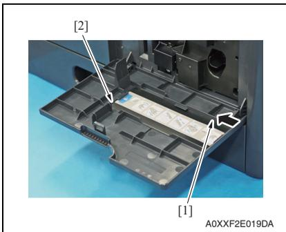
2. While releasing the tab [1], remove the front door [2].
