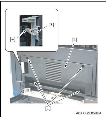
1. Remove four screws [1], and remove the fan motor cover [2].
