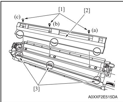
13. Remove three screws [1], and remove the developer scattering prevention plate [2].
