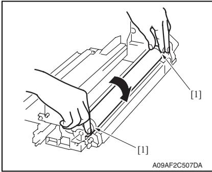
3. Hold both ends [1] of the drum with your both hands and turn the drum a half turn in the direction of the arrow.
