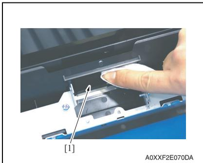
3. Using a cleaning pad dampened with alcohol, wipe the multi bypass tray feed roller [1] clean of dirt.
