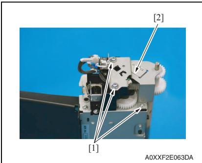
2. Remove three screws [1], and remove the fixed sheet metal [2].
