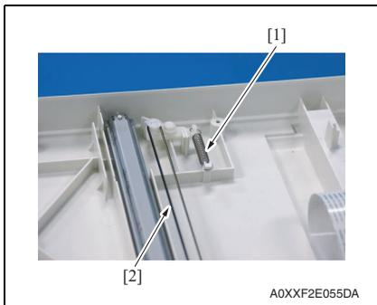
5. Remove the spring [1] to reduce the tension of the belt [2].
