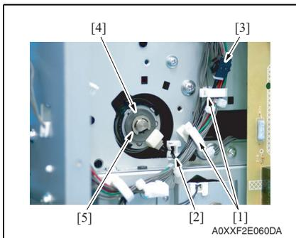
3. Remove the harness from two wire saddles [1] and edge cover [2].
