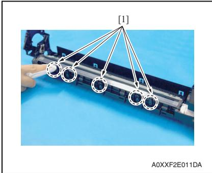
4. Using a cleaning pad with alcohol, wipe the five separator fingers [1] clean of dirt.
