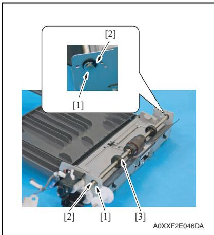
4. Remove two E-rings [1] and two bearings [2].
