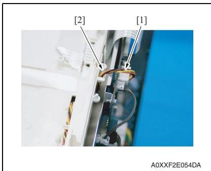
3. Disconnect the connector (P101) [1] on the printer control board.
