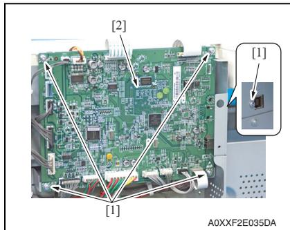
3. Disconnect all connectors from the printer control board.
