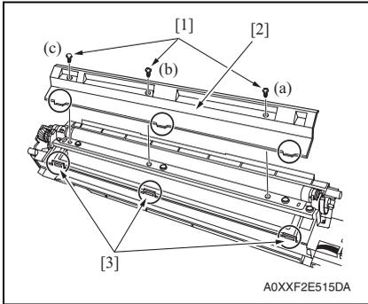
7. Remove three screws [1], and remove the developer scattering prevention plate [2].
