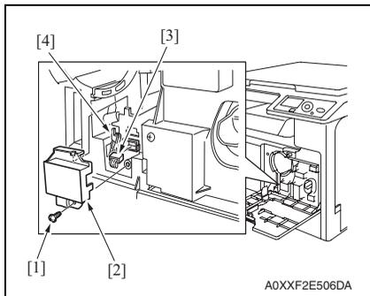
4. Remove the screw [1], and remove the cover [2].
