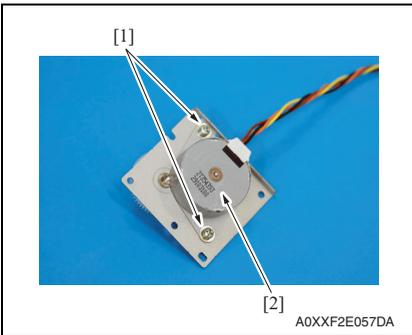
8. Remove two screws [1], and remove the scanner motor [2].
