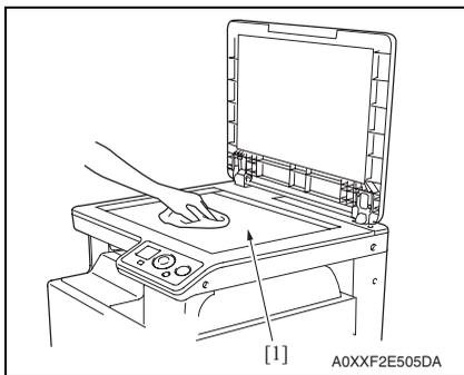
1. Using a cleaning pad, wipe the original glass [1].
