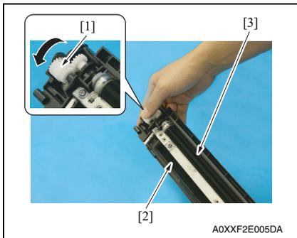
14. Tilt the developing unit as shown in the illustration. While turning the gear [1] in the direction of the arrow, dump the developer [2].
