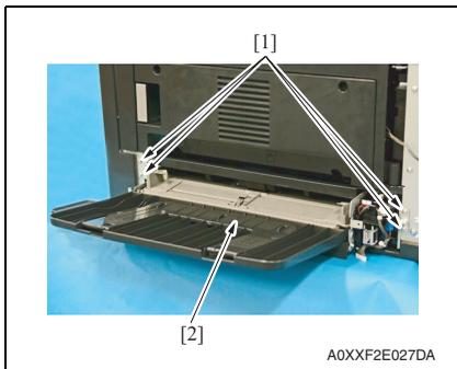
5. Remove four screws [1], and remove the multi bypass tray [2].
