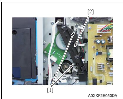
4. Remove two screws [1], and remove the harness guide [2].
