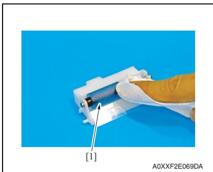
3. Using a cleaning pad dampened with alcohol, wipe the multi bypass tray separation roller [1] clean of dirt.
