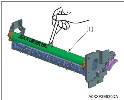
2. Using a brush, apply a light coat of toner to the surface of the drum [1].
