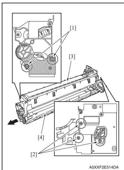
4. Remove two screws [1] in the rear of the imaging unit.
