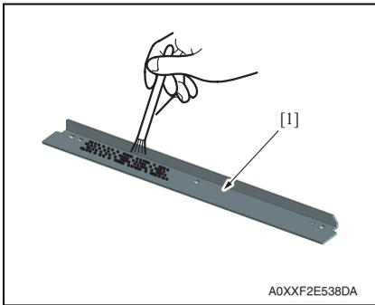
4. Using a brush, apply a light coat of toner to the surface of the cleaning blade [1].
