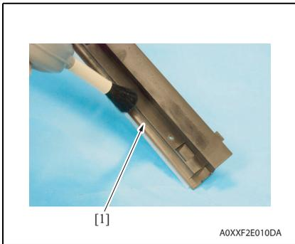
8. Using a brush, whisk dust and dirt off the surface of the developer scattering prevention plate [1].
