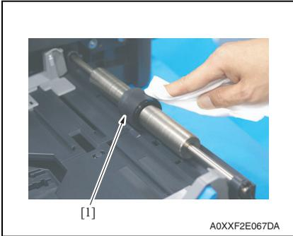
2. Using a cleaning pad dampened with alcohol, wipe the tray 1 feed roller [1] clean of dirt.
