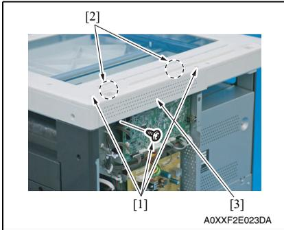
2. Remove three screws [1], and remove the scanner rear cover [2].
