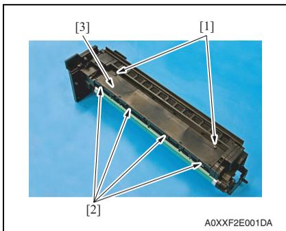
7. Remove two screws [1], release four tabs [2], and remove the plate [3].
