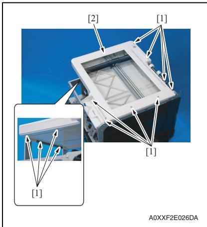
10. Remove twelve screws [1], and remove the original glass [2].
