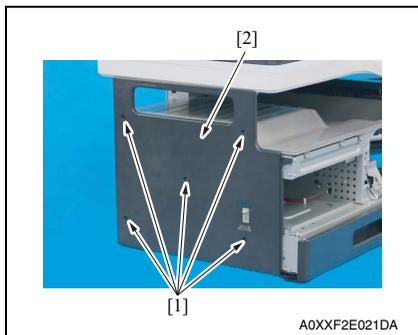
4. Remove four screws [1], and remove the left cover [2].
