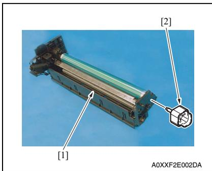
8. Turn the drum unit [1] over to place it as shown in the illustration.
