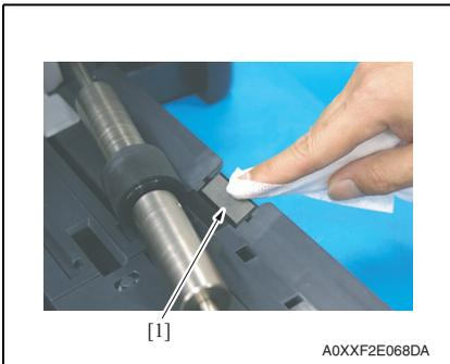
3. Using a cleaning pad dampened with alcohol, wipe the tray 1 separation pad [1] clean of dirt.
