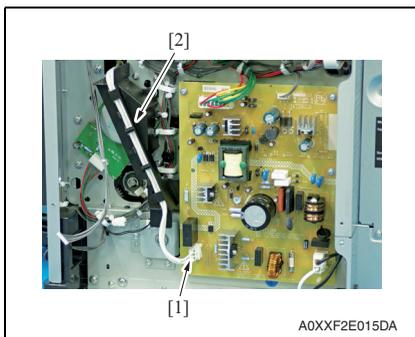
6. Disconnect the connector (CN2) [1] on the DC power supply.
