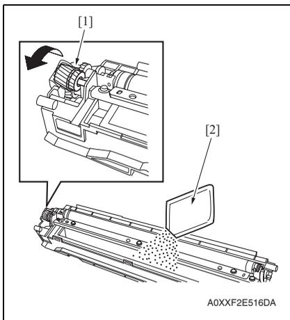
15. While turning the gear [1] in the direction of the arrow, pour a packet of developer [2].
