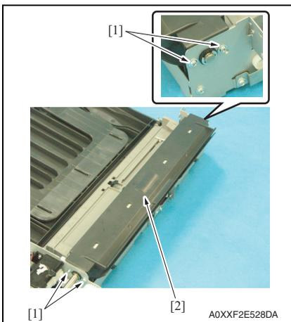
3. Remove four screws [1], and remove the multi bypass tray upper cover [2].
