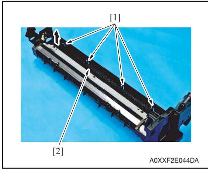
5. While releasing four tabs [1], remove the ozone filter [2].
