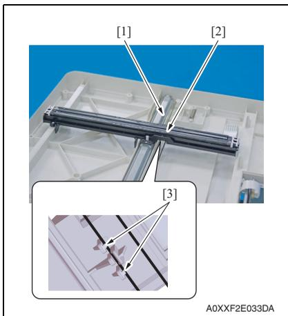
5. Remove the CIS module [2] from the belt [1].
