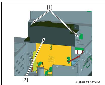
10. Remove two screws [1], and remove the paper exit inside cover [2].
