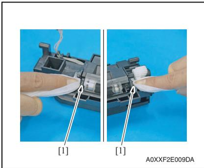
7. Using a cleaning pad with alcohol, wipe the two Ds collars [1] clean of dirt.
