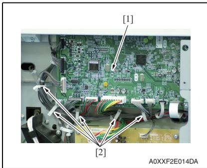
4. Disconnect the connector (P004) [1] on the printer control board.
