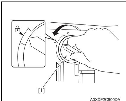
2. Rotate the empty toner bottle [1] counterclockwise to unlock it.
