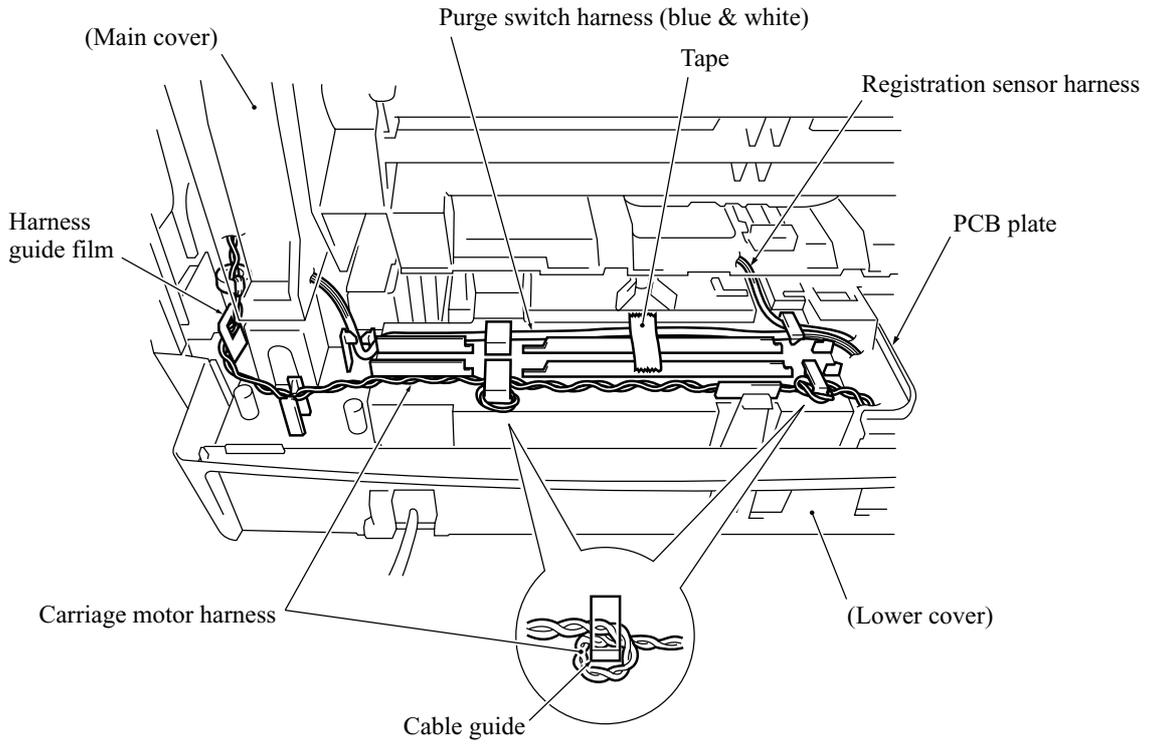
**Harness routing D: Purge cam HP switch harness and pump switching cam HP switch harness on the lower cover**
