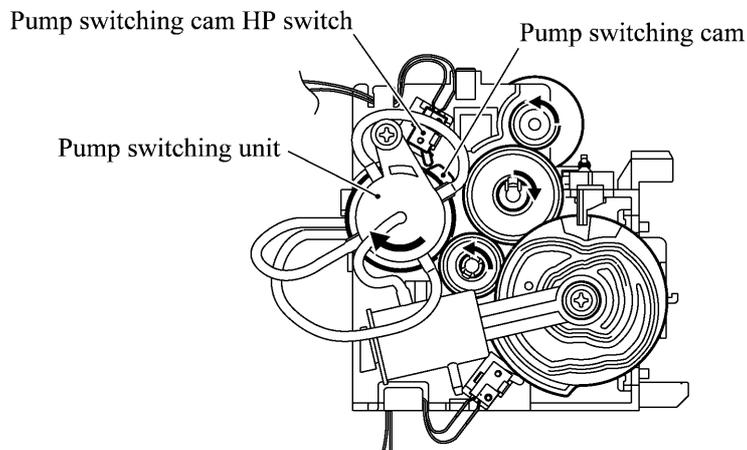
When the paper feed motor rotates clockwise
