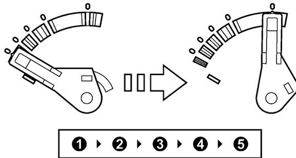
**NOTE:** Always turn the head adjuster lever in an ascending order. If you want to set the head adjuster lever to position 3, for example, turn it from 1 to 3. Once you have turned it to position 4, you need to turn it back to position 1 and then turn it to 3.
