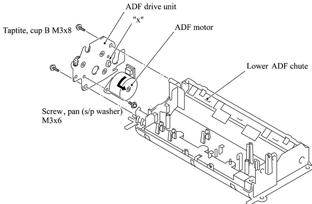
**Reassembling Note:** When setting the ADF motor, hook the non-screw side of the flange on section "x" (shown above) and secure it with the screw.
