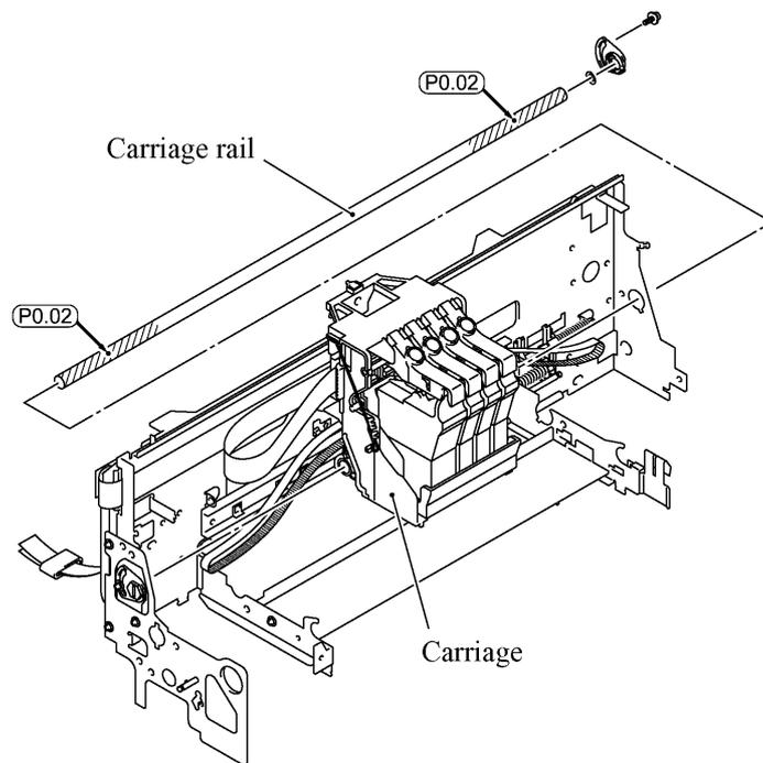
[ 8 ] Main chassis (slideway of the carriage guide)
