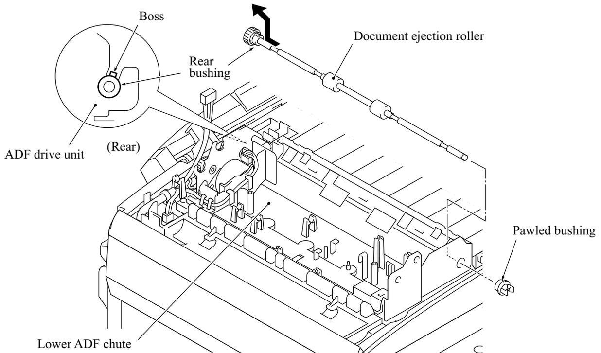
**Reassembling Note:** When fitting the rear bushing of the document ejection roller into the cutout of the ADF drive unit, orient the boss as illustrated on the previous page.
