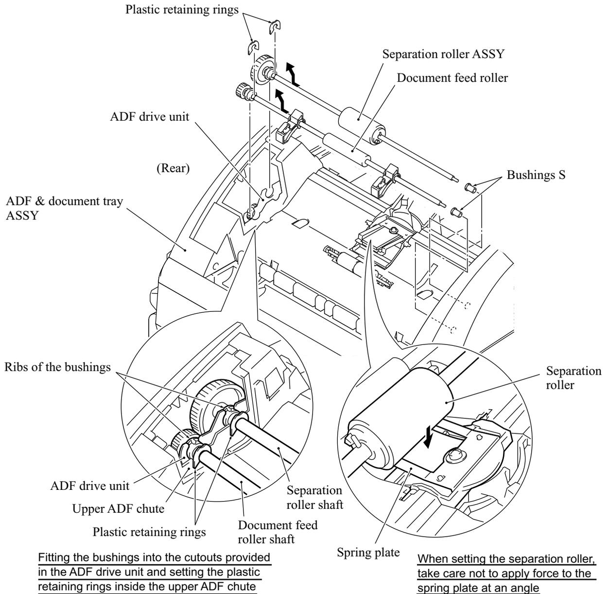
**Reassembling Note:** If you have disassembled the separation roller ASSY, set the separation roller on its shaft with the boss facing towards the pin and then snap the plastic retaining ring into place, as illustrated below.
