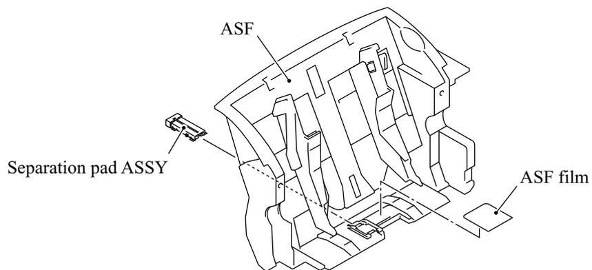
(4) Disassemble the separation pad ASSY as shown below.
