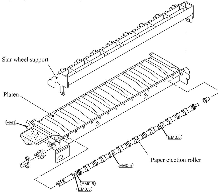
**[ 5 ] Paper ejection roller gear and PF roller gear**
