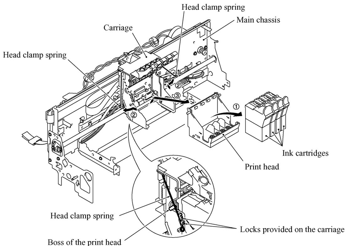
(2) Remove the head clamp springs as shown below.
