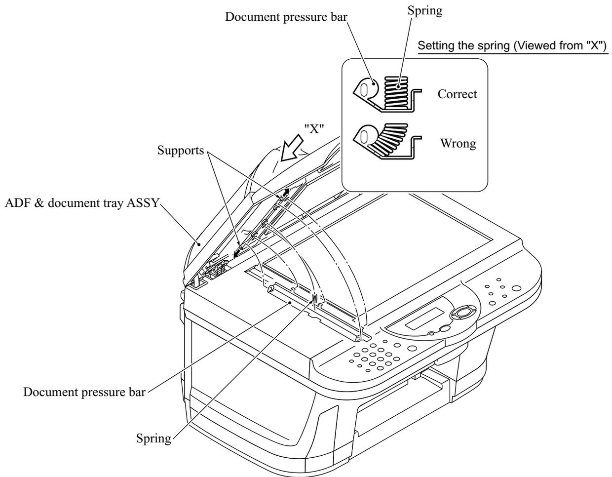
**Reassembling Note:** After setting the document pressure bar, check in the direction of arrow "X" that the spring is into place as illustrated above.
